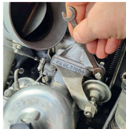
Nipping up the lock nut on the throttle stop after adjusting the idle
