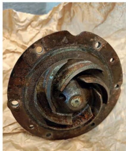
Old water pump was stiff, and corroded on sealing face
