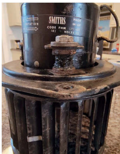
Ugly but strong - rubberised glue fixes bush and steadies motor
