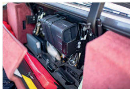
Part of the complex and sometimes troublesome power roof mechanism
