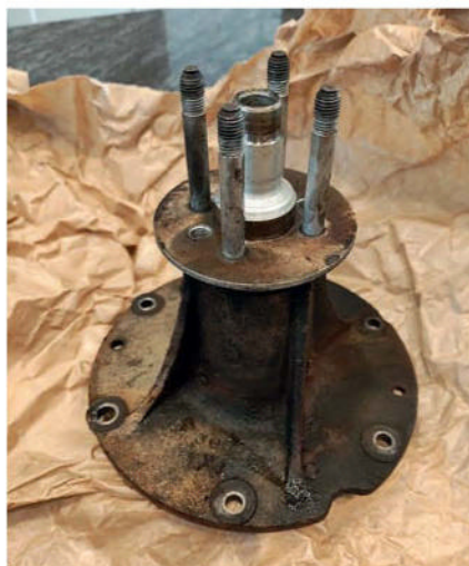
Any old iron? Failed water pump will go to Flying Spares to be remanufactured
