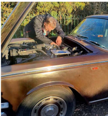
The distributor clamp bolt is tricky to reach
