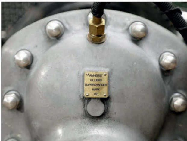
The 'Amherst Villiers Supercharger Mark IV' plate attached to the device on most 'Blown' Bentleys. Villiers had originally wanted much larger, more prominent branding.
